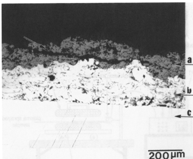
Fig. 3 Cross section of YPSZ coating system. The arrows indicate (a) Y_2O_3 (8 wt%) ZrO_2 TBC, (b) NiCoCrAlY bond coat, (c) nickel-chromium substrate, (d) macrocracking in YPSZ top coat. Differential interference contrast
